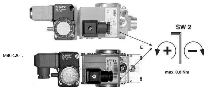
Figure 6: Diagram for setting the main volume throttle
